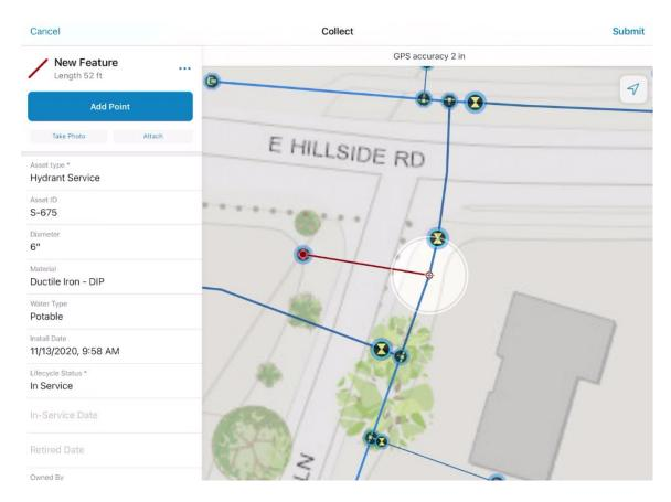
Figure 4. ArcGIS Field Maps lets users collect field assets in just a few taps and with high accuracy.
