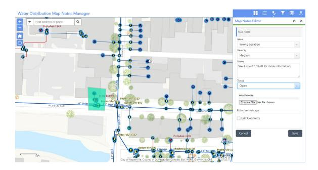
Figure 3. Water map notes allow field and office users to flag errors in your GIS data to ensure that your distribution system is accurately mapped.
